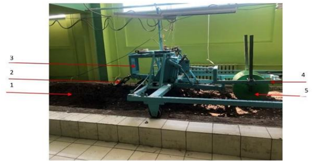
1 - Soil channel; 2 - traction dynamometer; 3 - movable cart; 4 - hitch; 5 - ice rink.
