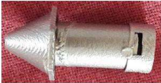
Fig. 8: The Developed Prototype of the Miniature Outer Casing of the Proposed Device 'MADE'
