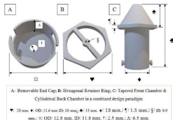
Fig. 7: Engineering Details of the Three Crucial 'Components of the Proposed Prototype MADE'
