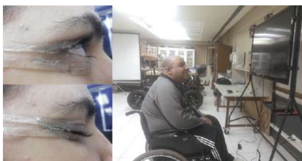
Fig. 12 Winkymote prototype using hydrogel
