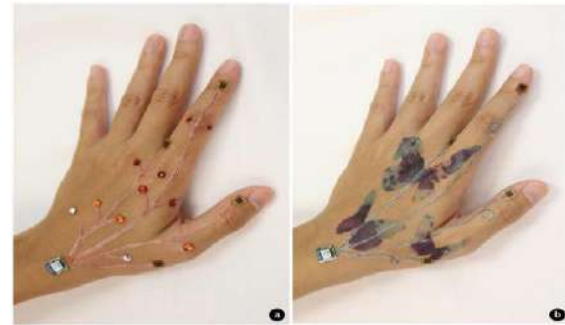
Fig. 5(a) Layout of the on-skin hand gestural interface Fig. 6 Aesthetic customization of Skin Wire devices with Explored in this paper (b) Implementation of Systemcolored wires and non-functional decorative elements such as (a) gems and (b) temporary tattoos
